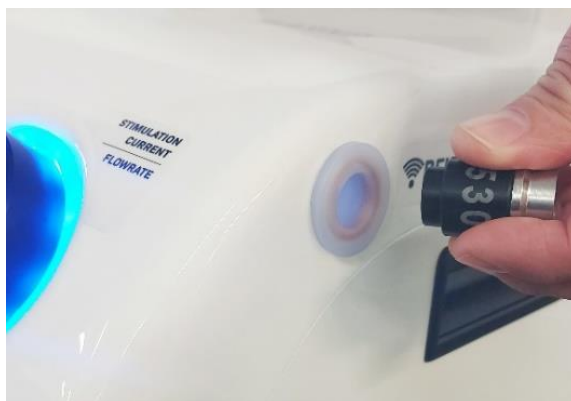
Fig. 10. Registration of the cryoprobe by means of the RFID tag
