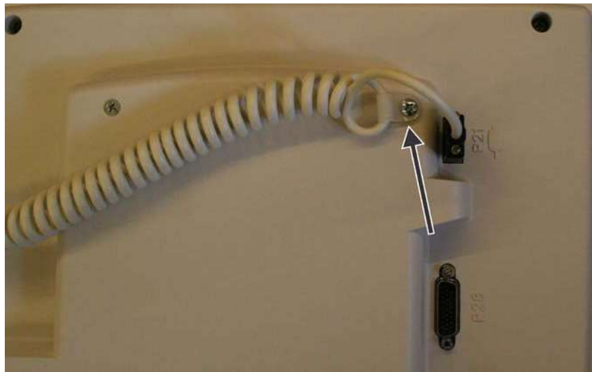
Figure 15 - 33: Use Clip to Attach Handswitch Cable to the Display Control Unit
