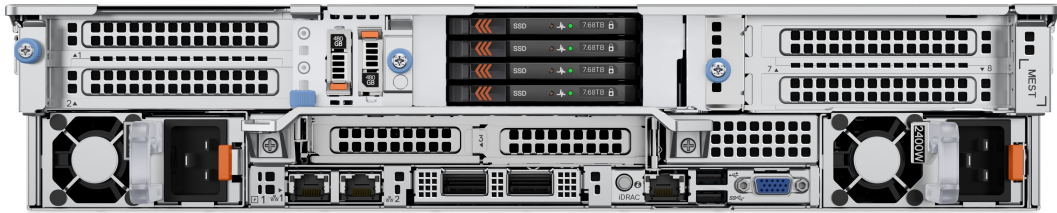
Figure 11. Rear view of the system with 4 x EDSFF E3.S rear drive module
