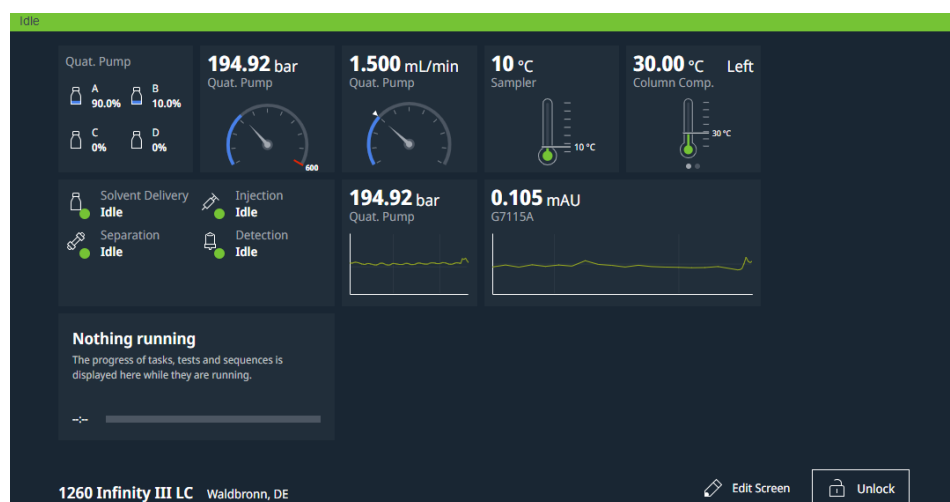
Figure 2. Ambient screen, displaying status information in customizable widgets.
