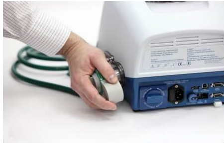
Figure 13 – Air/Oxygen Entrainment Mixer Installation
