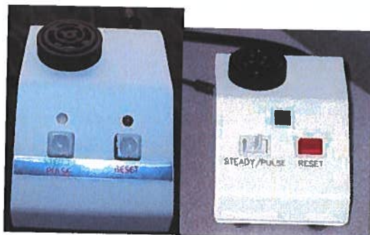
Figure 6-11 Patient Alert control box: Steady/Pulse button on left and Reset button on right
