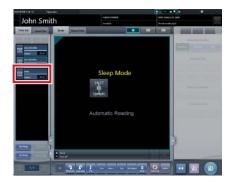
Added exposures are displayed in the exposure item list on the exposure screen ([Study List] tab screen).
