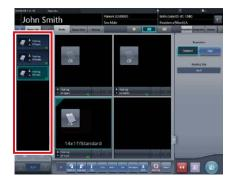
If you press the exposure conditions display area where the reading sequence of the examinations is specified, the specified reading sequence is cancelled.
