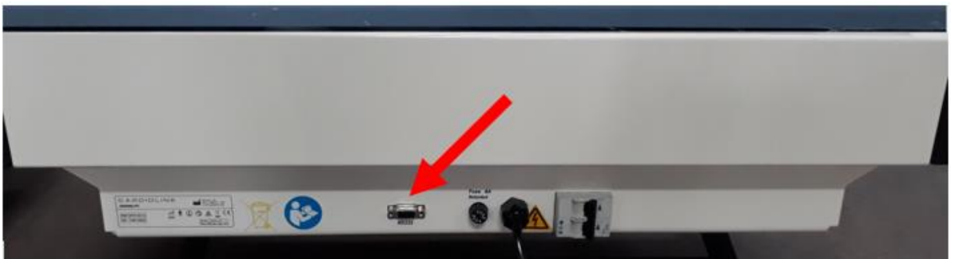
RS232 serial port positioning
