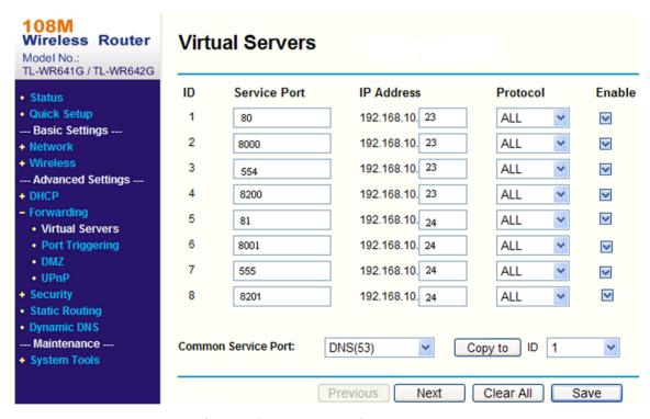
Figure 10-1 Port Mapping on Router
