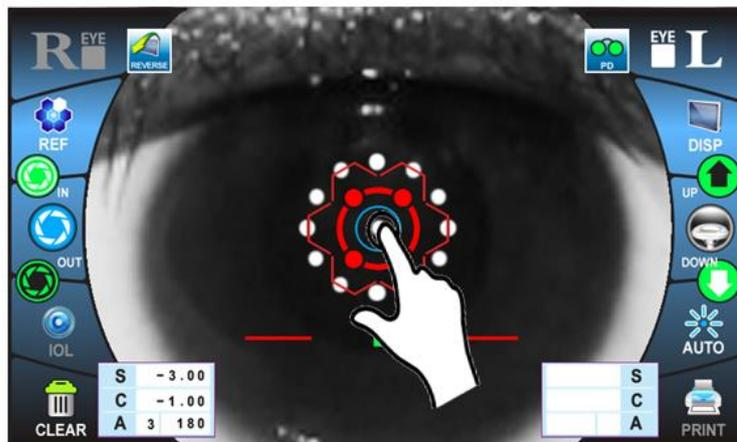
8) The instrument begins to measure, if the measurement button is pressed on the joy button after alignment.
