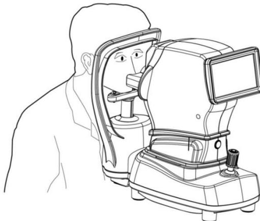
4) Adjust the chinrest height by touching "Chinrest Up/Down" icon or controlling the joystick until the patient's eyes are positioned on the screen.
