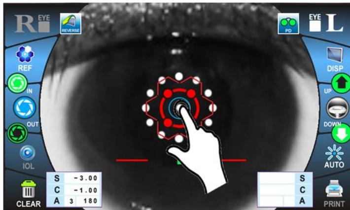
8) In a few seconds, the instrument begins to measure for times which is set on the MANU function.
