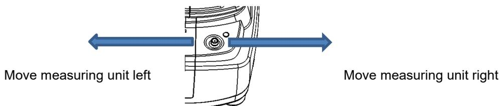
2) The position of measuring unit can be adjusted laterally by inclining the joystick to forward or backward with pressing joystick
