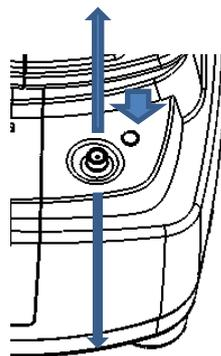
3) The position of measuring unit can be adjusted vertically by inclining the joystick to forward or backward.
