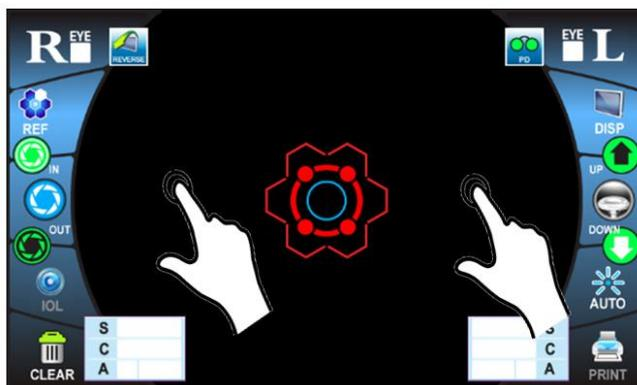
2) The position of measuring unit can be adjusted laterally by touching
