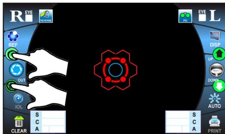
3) The position of measuring unit can be adjusted vertically by touching upper/bottom of touch panel.
