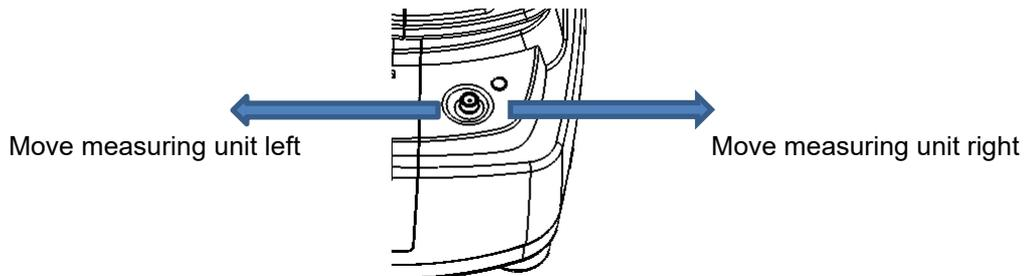
2) The position of measuring unit can be adjusted laterally by inclining the joystick to forward or backward with pressing secondary button
