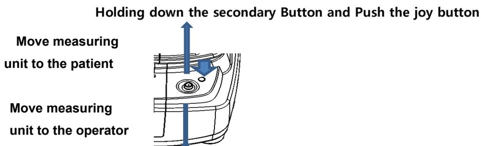
3) The position of measuring unit can be adjusted vertically by inclining the joystick to forward or backward.
