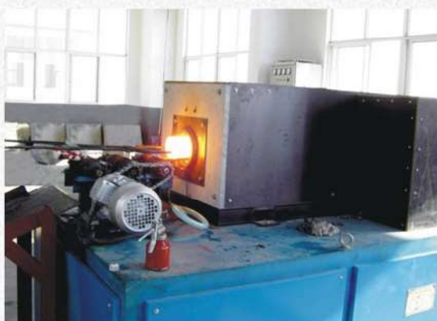
Induction heating cabinet with auto discharge device
