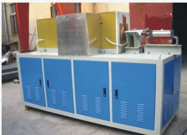
Induction heating cabinet-1
