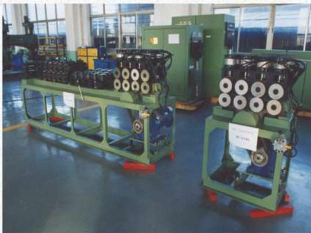
Straightening and hauling machine of Pipe pile steel wire heating treatment line
