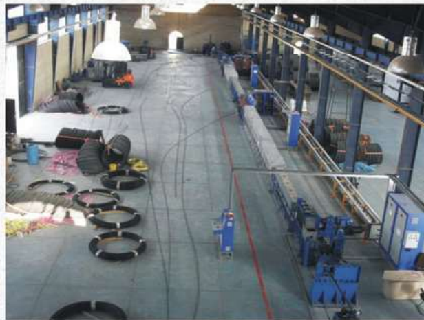
Spring steel wire heating treatment line on site
