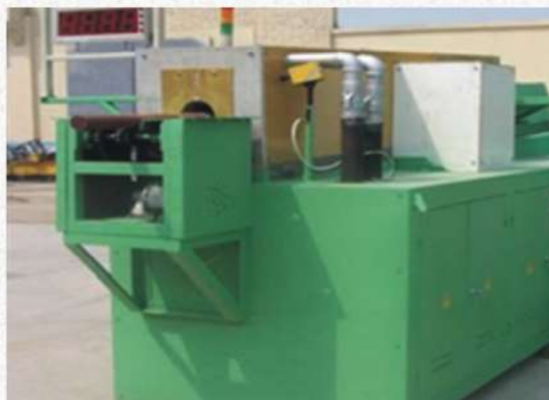
Induction heating cabinet with thermal detector and auto discharge unit
