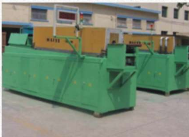
Induction heating cabinet with thermal detector and auto discharge unit
