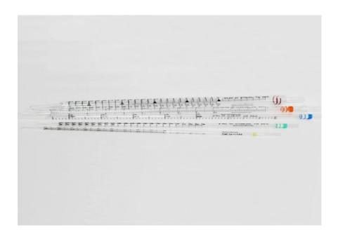
Serological Pipette, designed for quantitatively transferring and dispensing exact volumes of liquid. Manufactured from virgin polystyrene.
