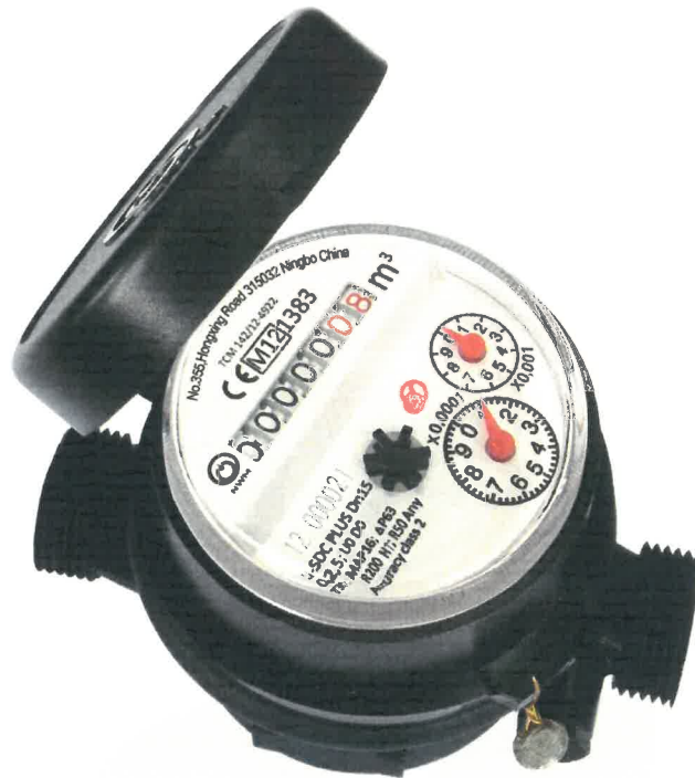
Figure 6: Example of dial plates of the water meter type SJ-SDC PLUS with 7+2, 5+4 and 8+1 registers. Variants with magnetic pointer for reed impulse transmitter or inductive pointer for AMR reading are also possible.
