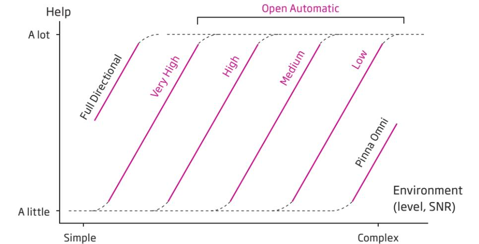
OpenSound Navigator directionality settings. In Pinna Omni, the hearing aid mimics sound as received by the human ear. In Full Directional, the focus is on sounds coming from the front. In Open Automatics, the hearing aid automatically adapts to the acoustical conditions, based on one of the four help profiles, Very High, High, Medium, or Low.
