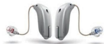
Oticon Opn S miniRITE uses the proven miniFit receivers and earpieces, fits up to 105 dB HL and is powered by a 312-battery.
