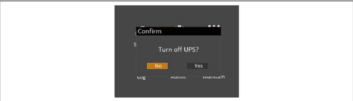
Figure 5.8 Bypass normal interface (Turn off UPS)
