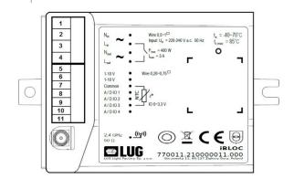
The iBLOC controller has a range of analogue and digital interfaces for controlling the lighting points. Available in the basic version or in a version with a power supply parameter meter. The user can either control the operation of luminaires via the analogue interface (the on/off function with a contactor, controlling light intensity with the 1...10 V protocol) or digitally via the DALI 2.0 interface.
