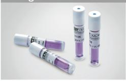
RENO SCBI (Self Containted Biological Indicator) is evidence for proper sterilization condition are achieved. Bacterial spores (Geobacillus stearothermophilus); Spore Population: 1.9 x 10<sup>6</sup> Spores / Unit.
