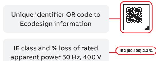
Unique QR codes are located on the rating plate and/or the front side of the drive.
