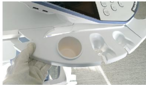
Figure 8-16: push button to remove the probe holder (e.g., at left side)
