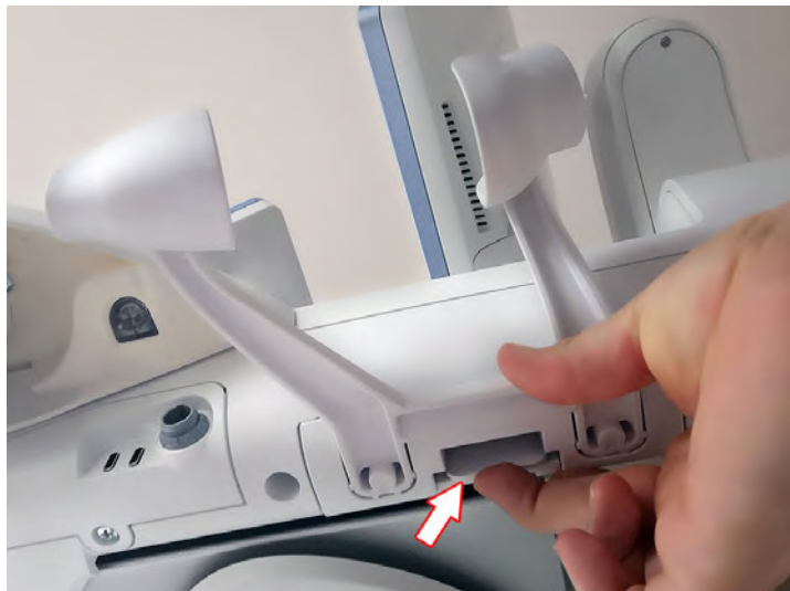
Figure 8-21: push against latch and pull the probe holder downwards
