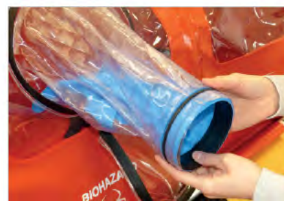
sleeves with gloves easy replacement of gloves, including cover cases
