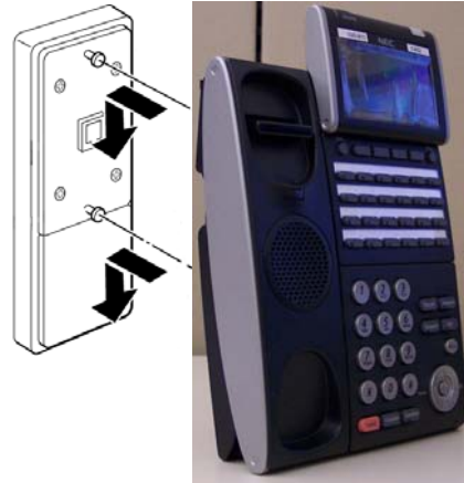
Figure 5-75 Wall Mounting Base on Switch Box
