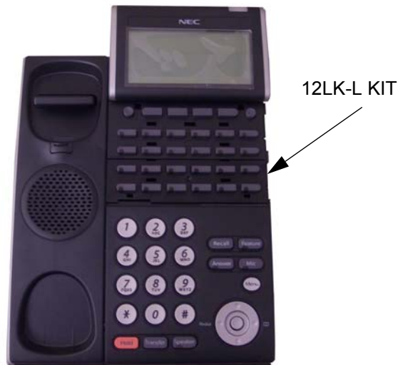
Figure 5-46 Installing the 12LK-L KIT
