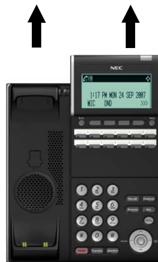
Figure 5-120 Removing the Multiline Terminal
