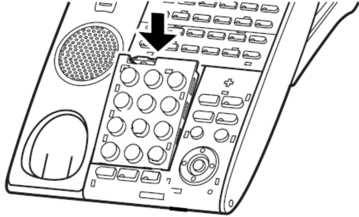
Figure 5-55 Install New Numbered Keypad into DT300/DT700 Series Terminal
