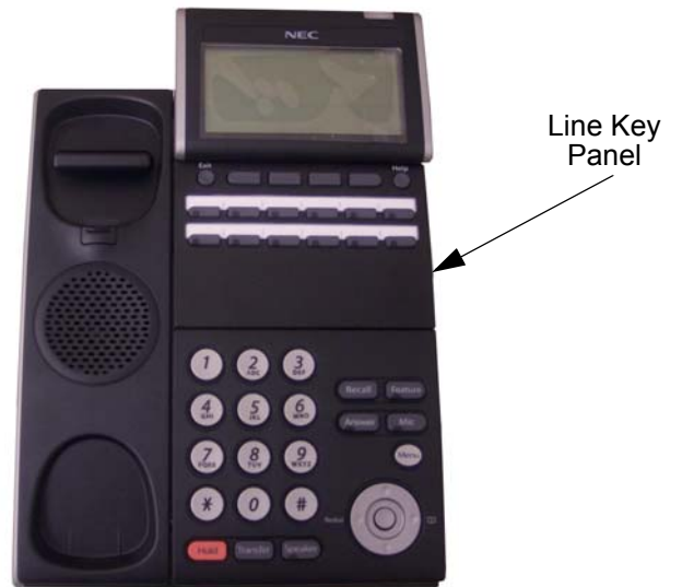
Figure 5-43 Removing the Line Key Panel
