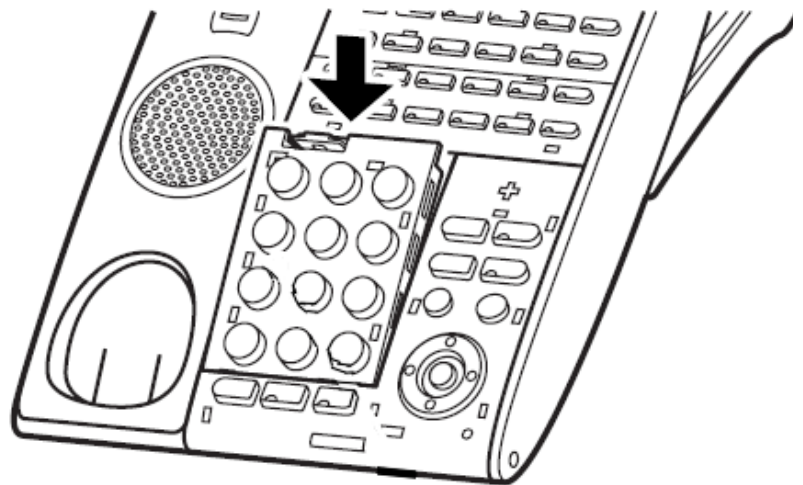
Figure 6-45 Install Numbered Keypad
