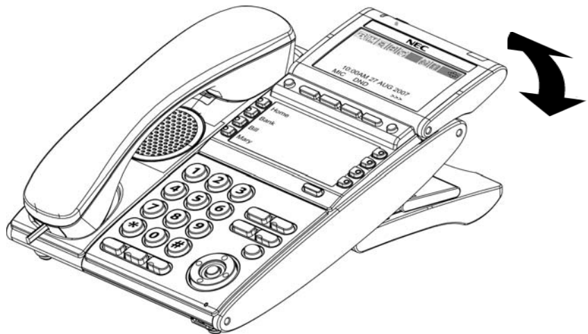
Figure 5-41 Adjusting the LCD on a Multiline Terminal
