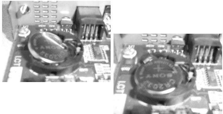
Figure 4-26 Install the CR-2032 Battery
