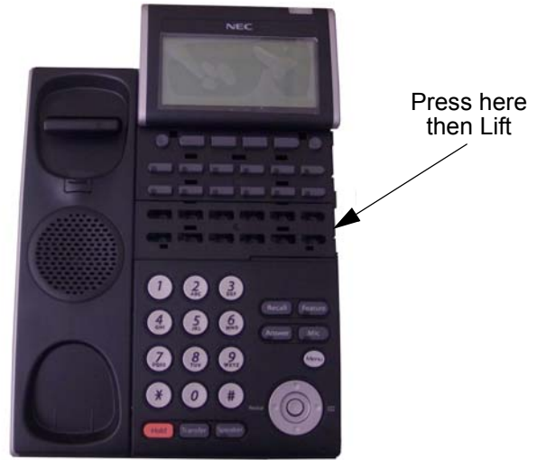
Figure 5-45 Removing the Line Key Placeholder
