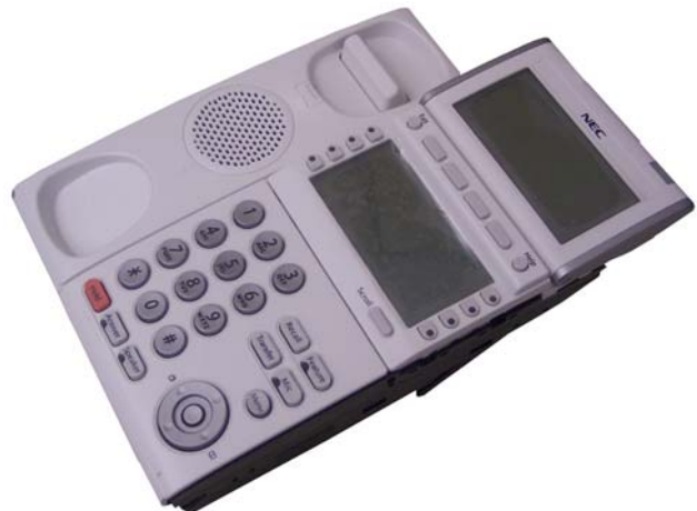
Figure 5-93 8LKD (LD)-L UNIT Installed
