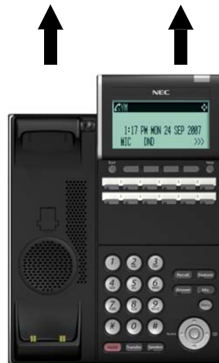
Figure 5-74 Removing the Multiline Terminal
