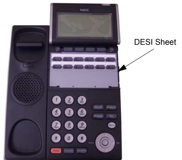
Figure 5-44 Removing the DESI Sheet
