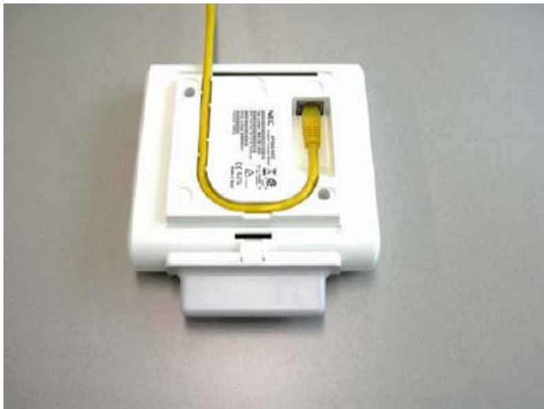
Figure 5-185 Install AP400 Base Station
