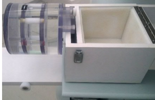
Figure 213. - Positioning the phantom
