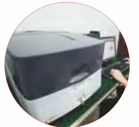
Energy dispersive X-ray fluorescence spectrometer To detect the harmful materials, according to the demand of EU standard
