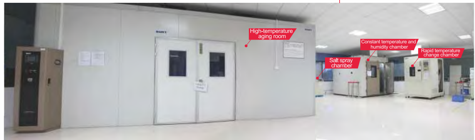
Climate Environmental Laboratory Simulate various extreme climate environments to ensure the quality of products.
