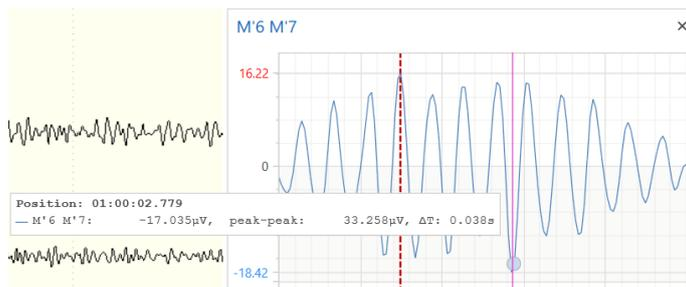
It is possible to double click to fix and compare two different values on the amplitude graph and in this case the active box will show information about the difference between the selected peaks:
