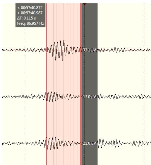
The area selected by the Standard Measure Cursor can be resized by clicking with the mouse on the start point (or on the end point) of the selection and dragging it to the desired position. The selection can also be moved by clicking with the mouse on the red area and dragging it to the desired position.
