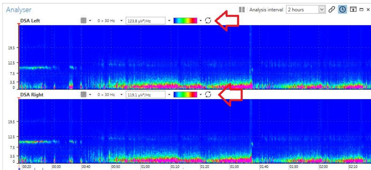
This toolbar allows the user to modify visualization properties for each Analyzer graph independently one from the others. From left to right:
