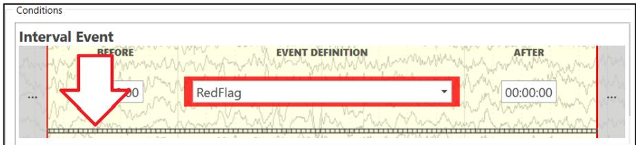
From Reduction tab it is possible to select one of the saved protocols to visualize on the open trace a **Preview** of the reduction that can be performed and to **Run** it to start the reduction. Reduction can be even launched from File Manager interface, right clicking on an EEG exam, and selecting “Reduce”. Available protocols are the ones defined in Brain Quick.
