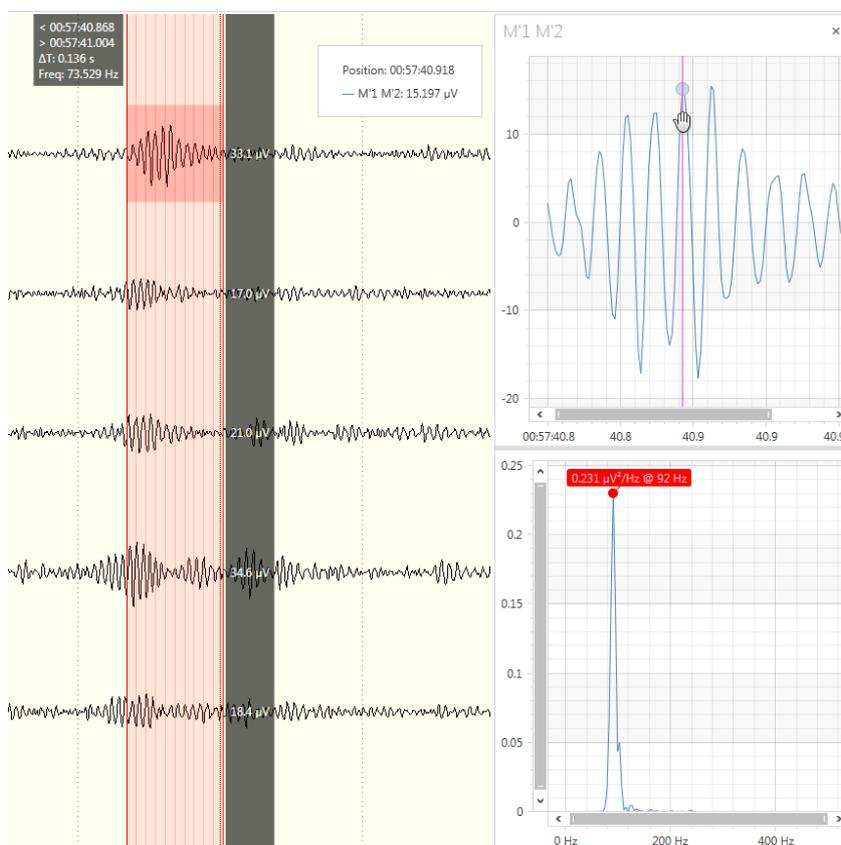
Hovering the mouse over the Advanced Measure Cursor's graphs the user can obtain additional information about the amplitude or the power of the trace: each graph provides a vertical cursor which is displayed when the mouse hovers on the plot. When the vertical cursor is active a box displays information about the position and amplitude of the selected point for the zoom graph and about frequency and power of the selected point for the spectrum graph.
