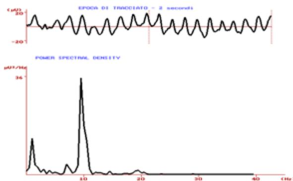
Frequency analysis consists in the segmentation of the EEG trace in multiple epochs of 2 seconds or more, transformation of each of these according to Fourier, then averaging the various spectrums and displaying the results obtained as a graph.
