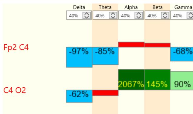
In the case of Power After lower than Power Before, the bargraph is blue. On the other hand, in the case of Power After higher than Power Before, the bargraph is green. Deep of blue/green colour depend of % of difference.
