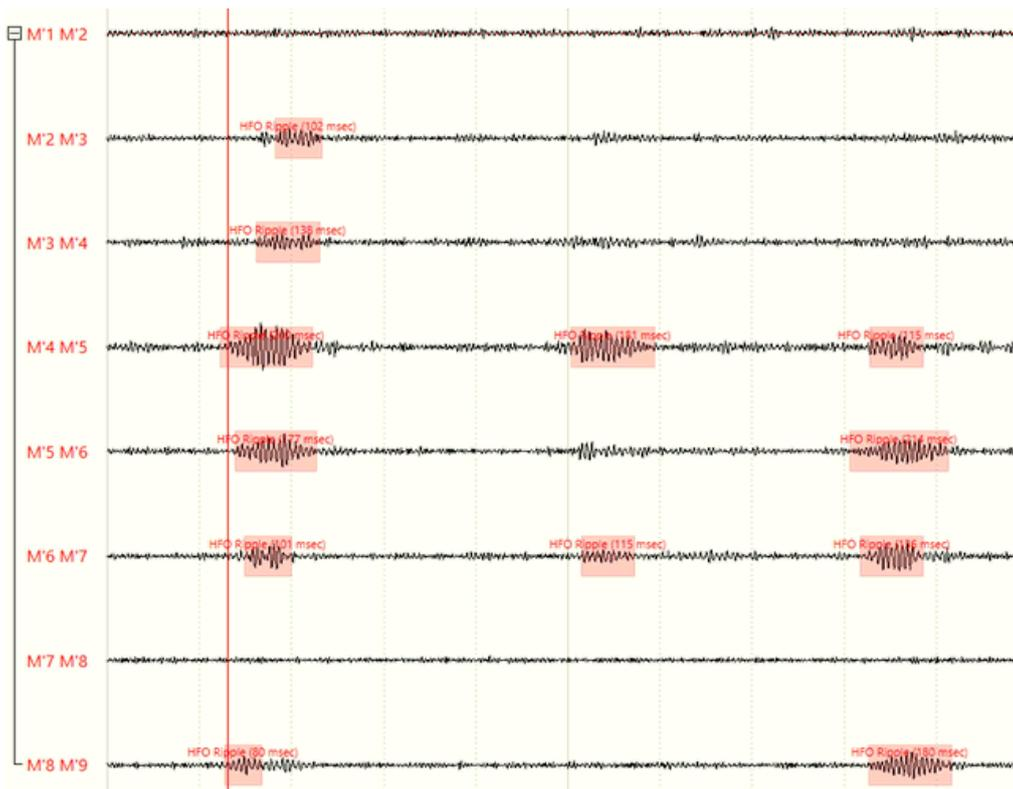
Figure: FIR Filter between [80-250Hz]
