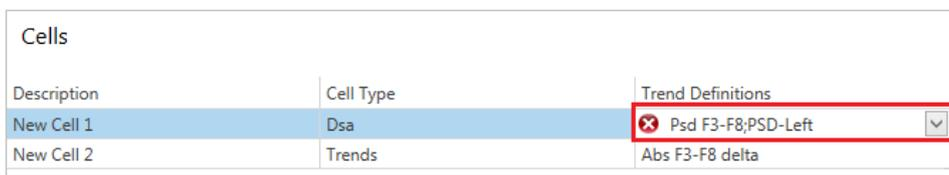
6. Select on Alert Threshold Type by clicking on **Alert Threshold Type** button. From this options it's possible to enable an alert if the analysis is inside or outside two bounds, above or below one threshold. Each Threshold are settable using Inferior and Superior Alert Threshold options.
