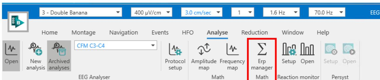
When clicking on the button, the Data Average directly opens on the right of the EEG page. It is composed of a new eeg window, which corresponds to the ERP Preview, and a panel with ERP Processing settings.
