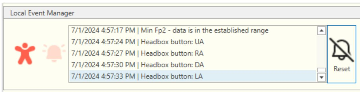
With the Local Event Manager window open, the software will prompt information regarding alarms during the recording of an EEG exam. Once an alarm is triggered, a sound will start playing to alert the user and a red flashing icon will appear to the left of the information box. No alarm will be issued if the current EEG exam is not currently been saved.
