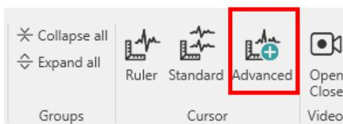
When clicking on the **Advanced** button the Advanced Measure Cursor directly opens in the middle of the EEG page. It is composed, as the Standards Measure Cursor, of a red area that delimits the part of the EEG trace to be measured. The selection applies to all the montage lines and by default the first montage line is selected.
