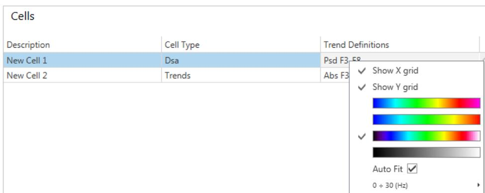
**NOTE:** color scale and frequency scale properties are available only for cells with type Dsa.
