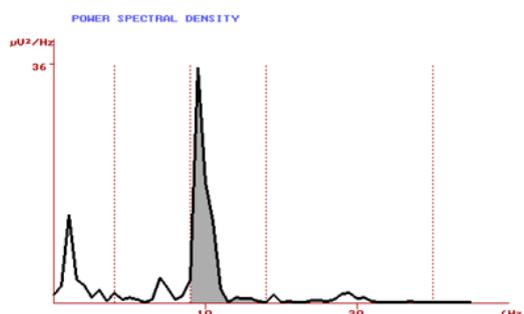
Absolute power of the Alfa band shown as a shaded area of the spectrum.
