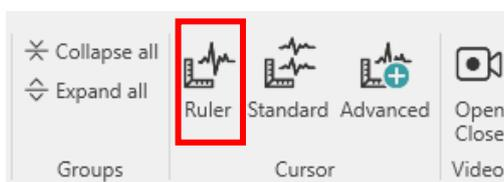
A floating ruler with graduated axis appears when hovering the mouse on the EEG trace. The ruler can be positioned in correspondence with the oscillations of interest to measure their amplitude and it can be fixed on the EEG page using shortcut CTRL+F and unfixed using again CTRL+F.
