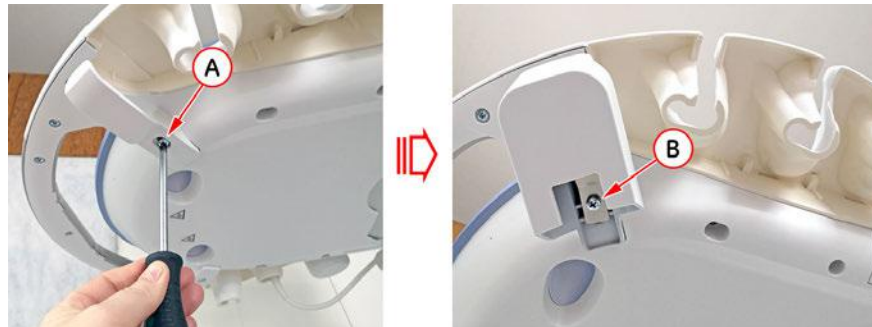
Figure 8-29: exchange cable hook
