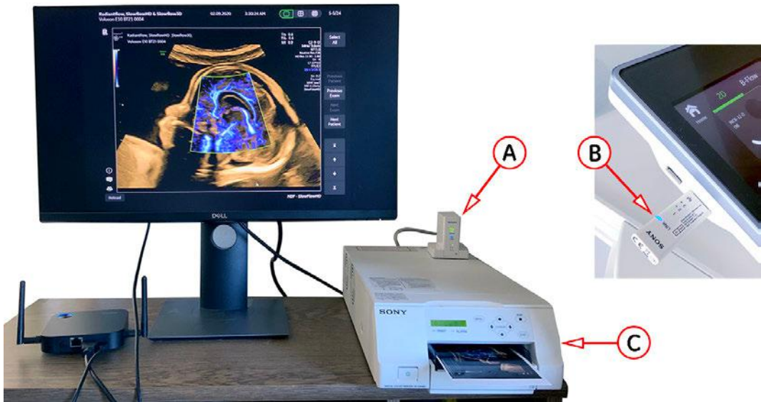
Figure 8-26: Example: Color Printer connected by means of Wireless Kit
