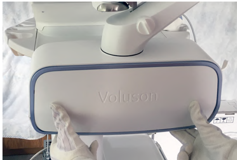
Figure 8-14: remove Rear Cover Top
