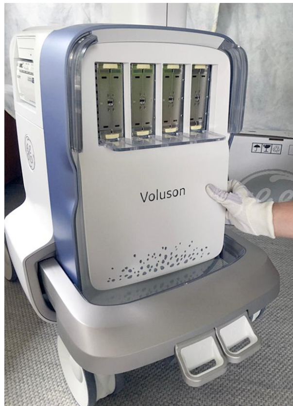
Figure 8-15: remove Front Cover
