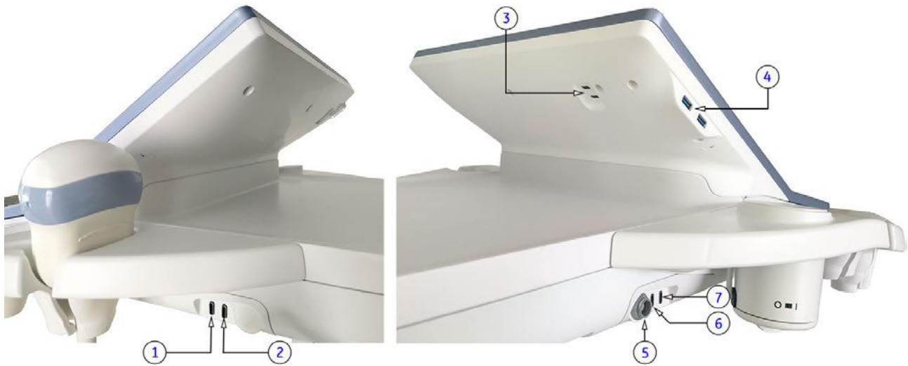
Figure 3-69: External I/O connectors - back and left/right side of the console
