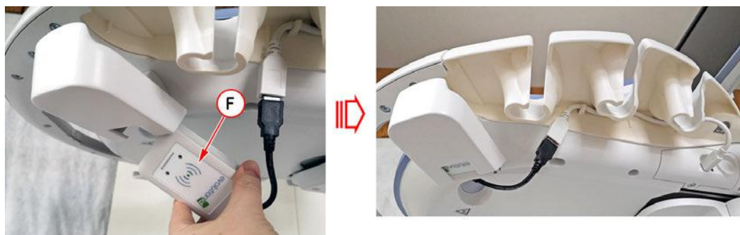
Figure 8-31: mount the RFID Log-on reader
