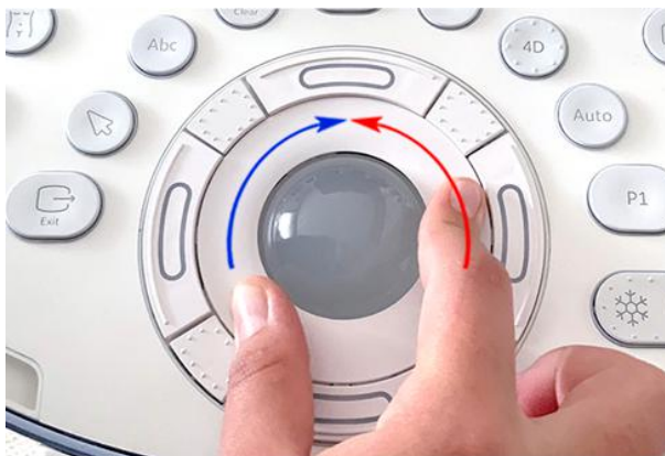
Figure 8-22: Trackball with Trackball "fixation" ring
