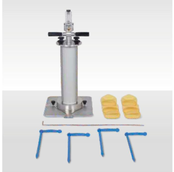
NF Type Balloon Density Apparatus are supplied complete with complete with;
