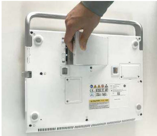
Figure 3-10. Put the battery into battery box
