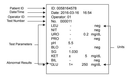
Depending on the type of strip selected, the analyzer recognizes the parameter order and automatically ranks the display and printing sequence of each parameter. Arbitrary results will always be printed automatically. Conventional or SI results will be printed based on the units selected. Abnormal results, or results of pathological significance will be marked with an \*.
