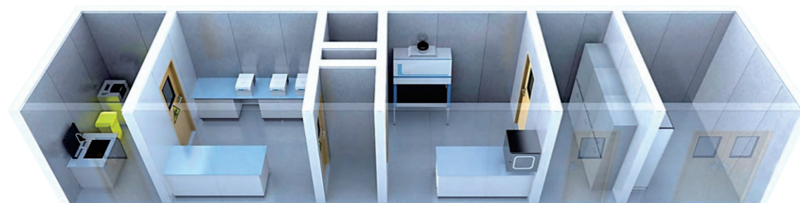
Decontaminating room Nucleic acid detection room Buffer room Sample processing room Machine room Dressing room
