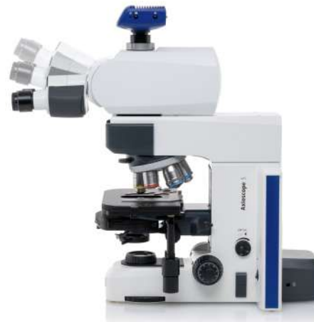
Ergophototube with 25 mm FOV and a tilting range from -2 to +28°. Also suitable for coobservation setups.
