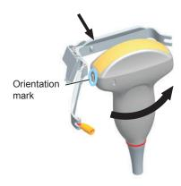
6. Attach the biopsy bracket to the probe and fasten the biopsy bracket with the locking screw.
