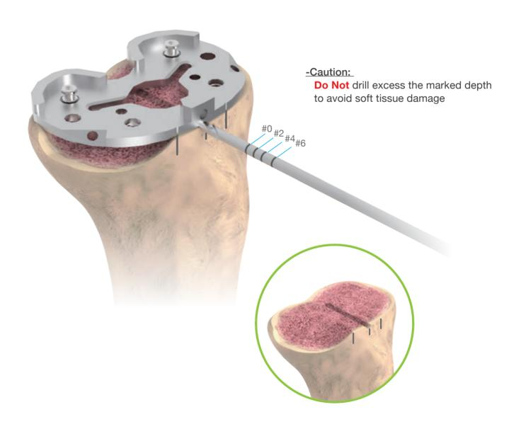
Assemble the appropriate **Tibial Augment Resection Guide** (left or right) and the **Tibial Augment Resection Guide Adaptor** onto the **Tibial Baseplate Trial**.
