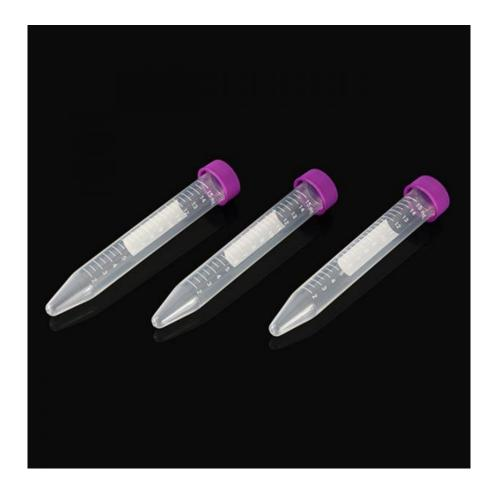
Sterile polypropylene centrifuge tubes are compatible with various standard rotors.
