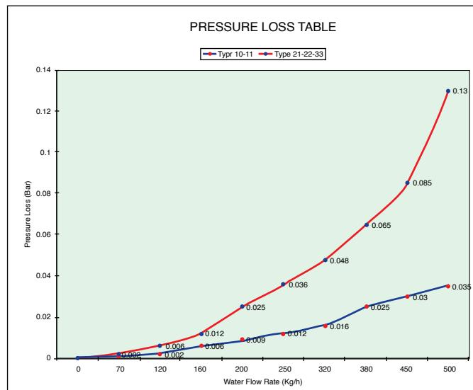
**Example:** What is the pressure loss on a 600/22DPDC/1000 radiator?
