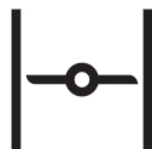
Electromechanical discharge valve
