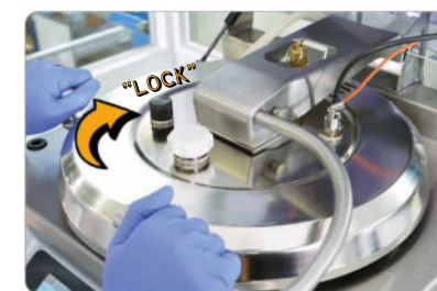
Safety lock with 12 hooks !
