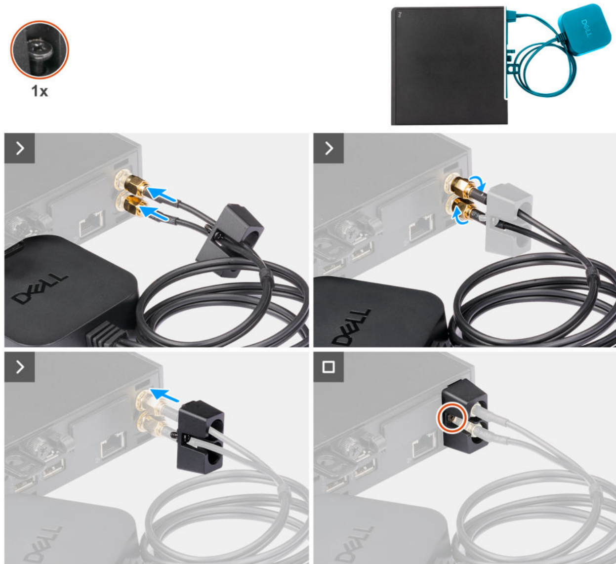
Figure 35. Installing external puck antenna
