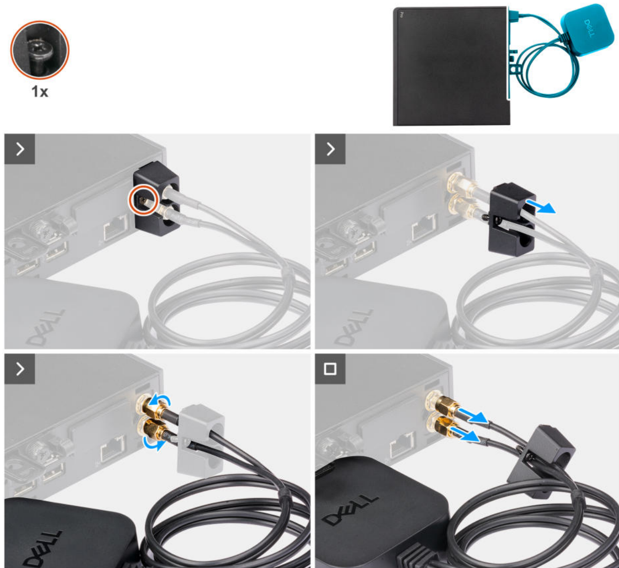
Figure 34. Removing external puck antenna
