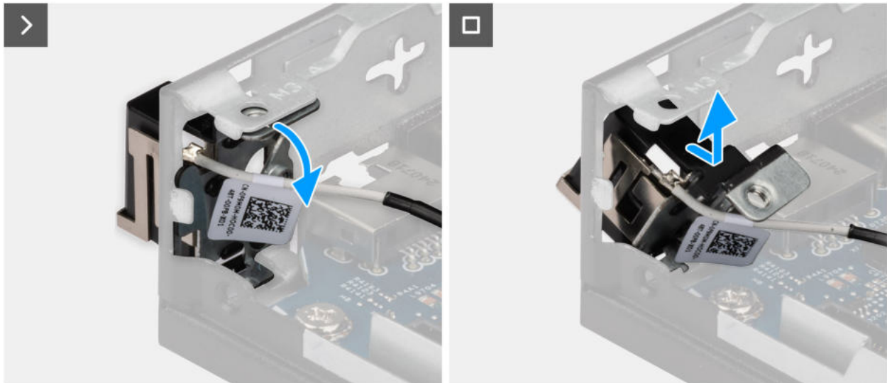
Figure 73. Removing the antenna module (white cable)
