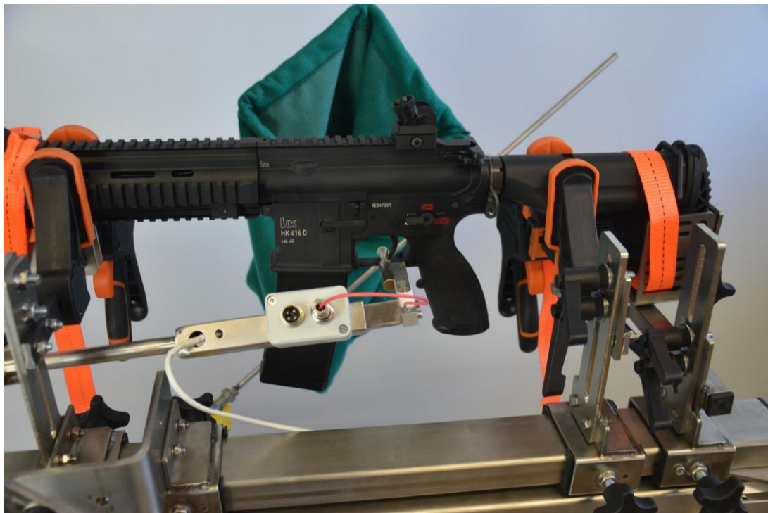
Fig. 14 - Adjusting the trigger actuator to the weapon
