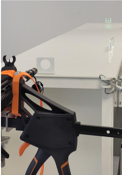
Fig. 11 - Positioning (aiming) the weapon through the catcher's sights
