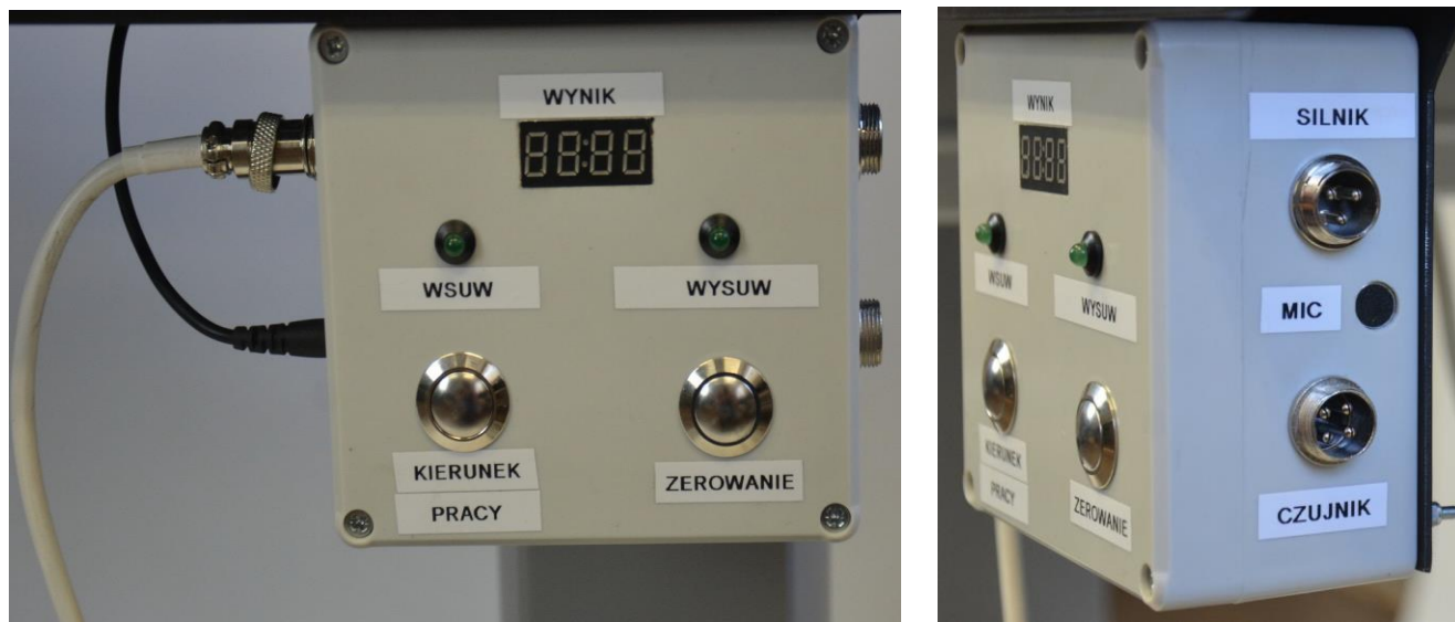
Fig. 4 - View of the trigger pressure actuator controller and trigger force measurement
