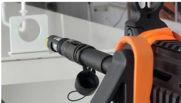
Fig. 3 - Mounted laser pointer with magnet on the barrel tip
