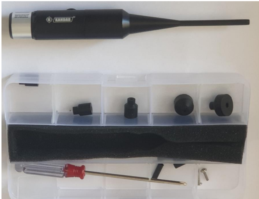
Fig. 8 - Laser pointer for weapon alignment with a magnet (weapon firing)
