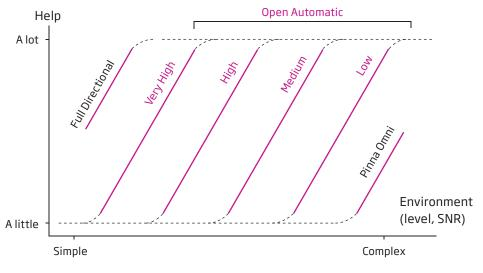
OpenSound Navigator directionality settings. In Pinna Omni, the hearing aid mimics sound as received by the human ear. In Full Directional, the focus is on sounds coming from the front. In Open Automatics, the hearing aid automatically adapts to the acoustical conditions, based on one of the four help profiles, Very High, High, Medium, or Low.
