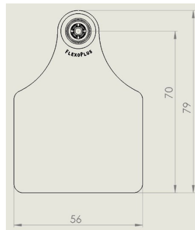
FlexoPlus D, mother part, dimensions
