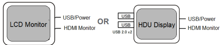
Figure 5-16 Top Console Block Diagram
