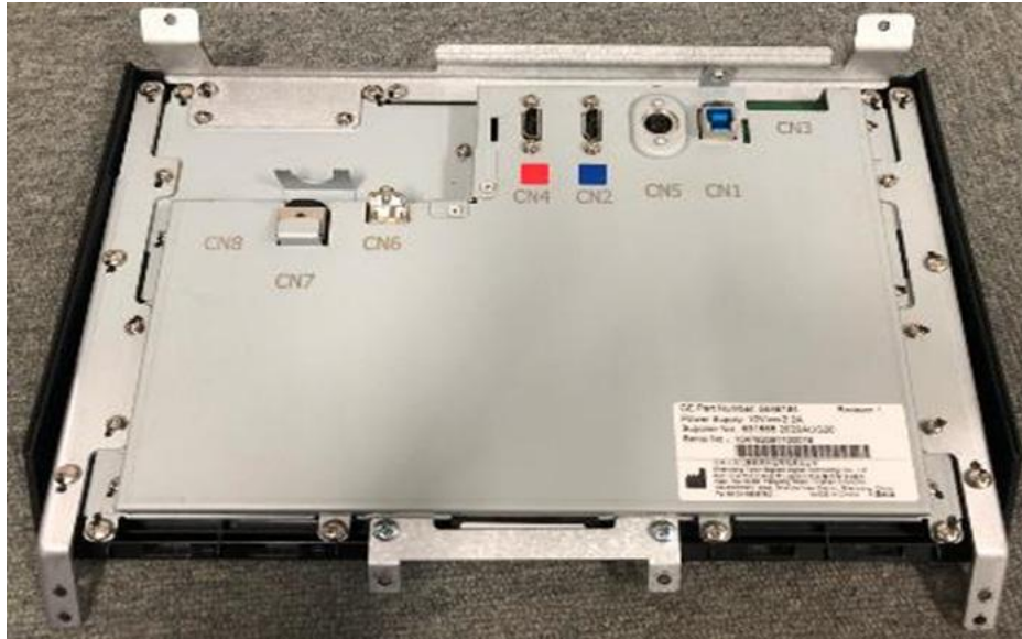
Figure 5-22 Upper Op Panel/Touch Panel Assembly Connections
