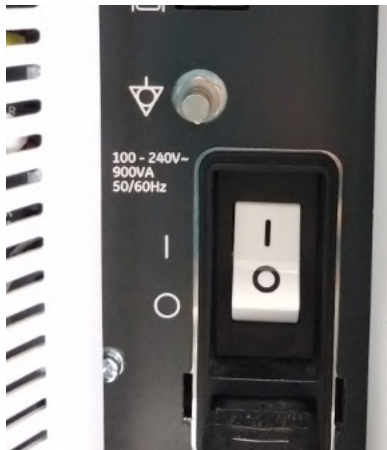
Figure 10-2 LOGIQ Fortis Main Power Supply Grounding Point
