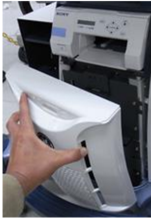
Figure 10-3 Remove the front cover
