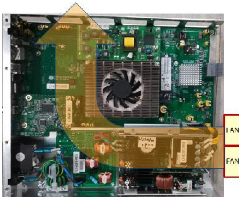
Figure 5-25 Cooling Air Flow of Power Supply
