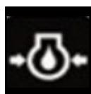
**Engine Oil pressure Low** - When engine oil pressure goes below 1.5 bar needle of the gauge moves to red band and the engine gets switched off.
