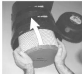
7 Place the OptiAir® cover back on the housing. Make sure dust ejection valve is orientated downwards.
