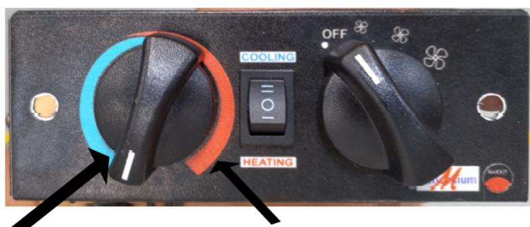
Mode Switch Must Be In Down engaged position For HEAT Mode
