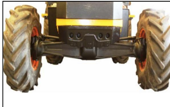
On two wheel drive machines the front axle is known as the steer able axle or dead axle. The axle is connected with a single horizontal centre pivot. This helps the front wheel to rise up and down while the machine is travelling in an uneven ground to keep the machine and its load level.
