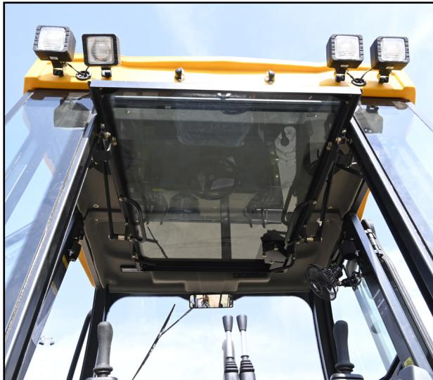
When the backhoe is shoved across the back of the machine and the bucket closed as shown in figure, the rear window can hit the bucket teeth (see warning below) If the backhoe is in position, move the Bucket clear before closing or opening the rear window.
