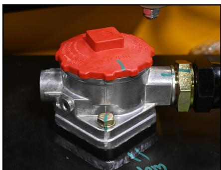
**Hydraulic filter element choke Indicator (C):**
