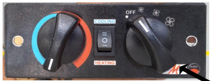
Mode Switch Must Be In up engaged position For AC Mode
