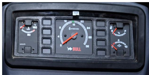
**Note :** If any of the working lights are "ON" while the engine is running, stop the engine as soon as possible. Do not use the machine until the fault has been rectified.
