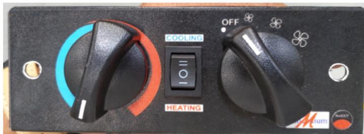
Mode Switch Must be in Middle engaged position for OFF
