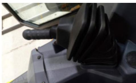
7. Move the machine by moving the dipper out while lowering the boom
