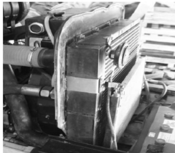
**Note:** If necessary, tilt the oil cooler away from the radiator to remove dust and debris between the radiator and oil cooler.
