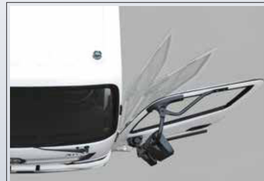
Reinforced doors gradually opening to 90°
