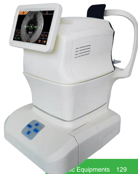
Corneal thickness measurement Auto soft air puff
