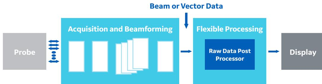
Figure 1. A traditional beamforming architecture.
