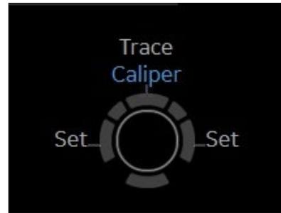
3. Place the second caliper in the appropriate location and press the “Set” right or left trackball key
