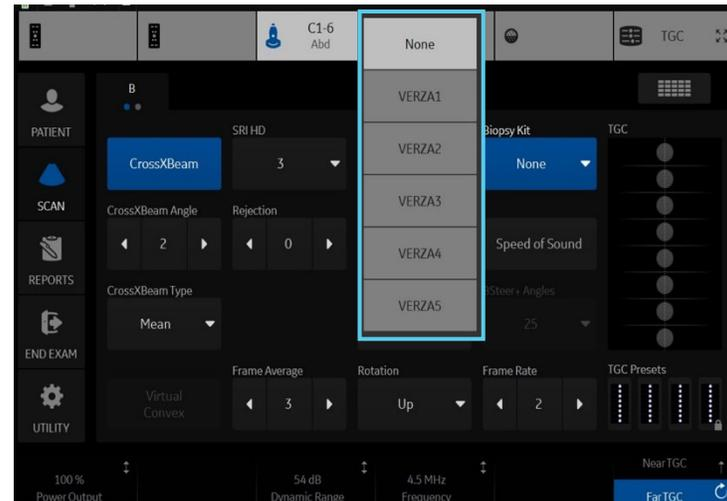
2. Select desired guide. Name and biopsy lines will show up on the screen. Be sure to match the number chosen on the screen with the number on the guide
