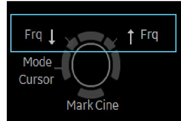
To configure the “Frq” keys, press Utility, System on Touch Panel, then User configurable key to choose the User Defined Trackball Set Key.
