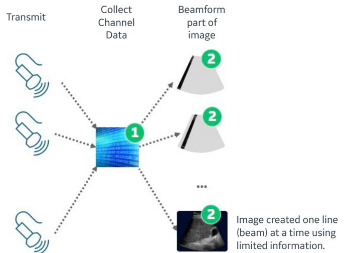
The channel data processed in step 2 and then overwritten still has useful information. However, a traditional beamformer has no means to extract this additional value before the channel data associated with the next transmit event overwrites it.
