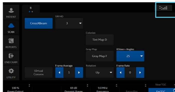
To display ALL touch panel parameters, select quick button on top right corner
