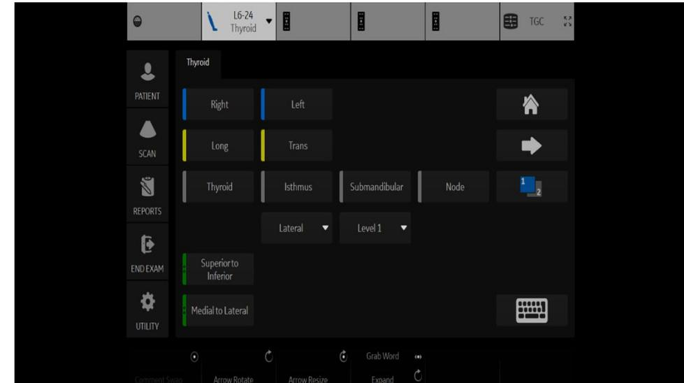
To select the comment cursor “home” position, move the cursor to the desired position. Push and hold the Home icon on the touch panel. The message “Set new home position” will be displayed on the bottom of the monitor.
