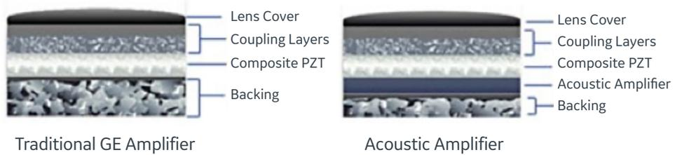
Figure 12. *Acoustic Amplifier*: Preserves the acoustic signal through an innovative design that captures and redirects the unused energy that passes through the crystal to enhance sensitivity, axial resolution, and penetration.
