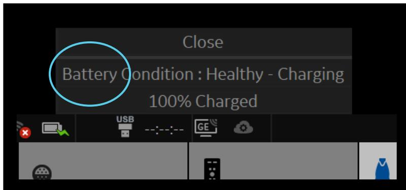
To check the percentage of battery life before disconnecting from AC power, click on the battery icon on the bottom left of the monitor.
