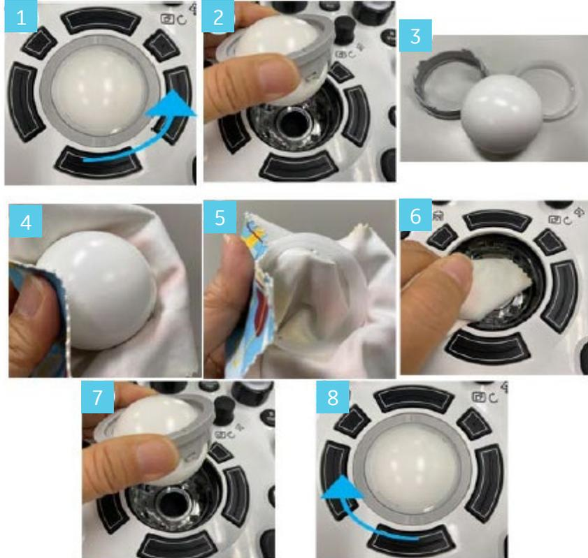
1. Twist and remove the trackball prior to cleaning the trackball and the trackball housing (1-3)
