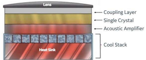
Figure 13. *Cool Stack*: Optimizes energy usage via patented technology integrated into the transducer’s internal architecture; it relieves inherent heat generation that can otherwise reduce sensitivity and penetration.
