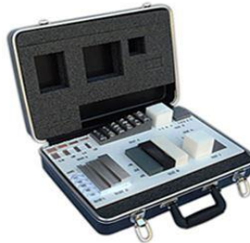
Figure 31: ASTM F792-08 Step Wedge (ASTM)
