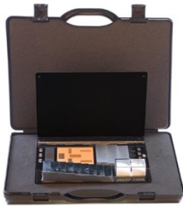
Figure 30: Exposed Wire Standard Test Piece (EW STP)
