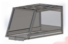
Smooth walls from 3 mm. thickness ST 52 or equivalent material with suitable reinforcements all around. Front frame with strong beams to stand thrust of hydr.-cylinder for the push-out-plate.
