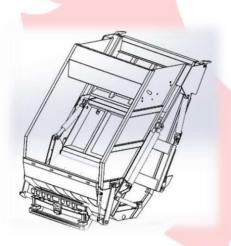
Tailgate connected to body with top hinges. The tailgate structure is consist of 1 sledge, 1 shovel, hopper and their cylinders. When garbage is put inside the hopper, with the help of the sledge and shovel this garbage goes into body and compressed with pushout plate. Sledge moves linearly and shovel moves radially to sweep the garbage inside the body, the sledge runs on sliding rails with roller or shoes.
