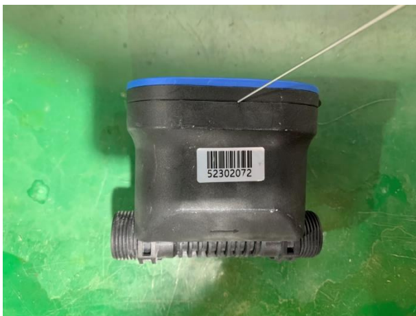
Fig 5: IP6X test (The wire of 1, 0 mm \Phi test of the IP6X) (The wire cannot penetrate the enclosure)
