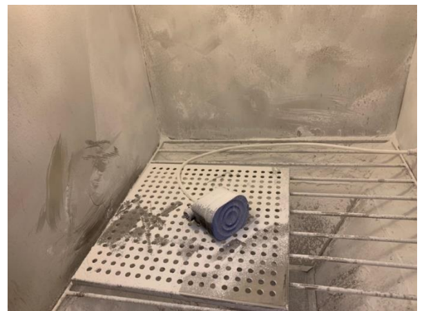
Fig 4: After the IPX8 test (No water in the shell. The battery has been filled with glue.)
