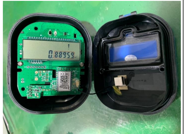
Fig 4: After the IPX8 test (No water in the shell. The battery has been filled with glue.)
