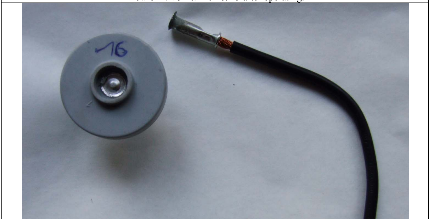
View of NNO 10/440 no. 16 after operating.
