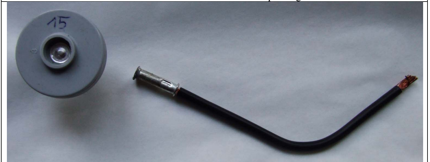
View of NNO 10/440 no. 15 after operating.
