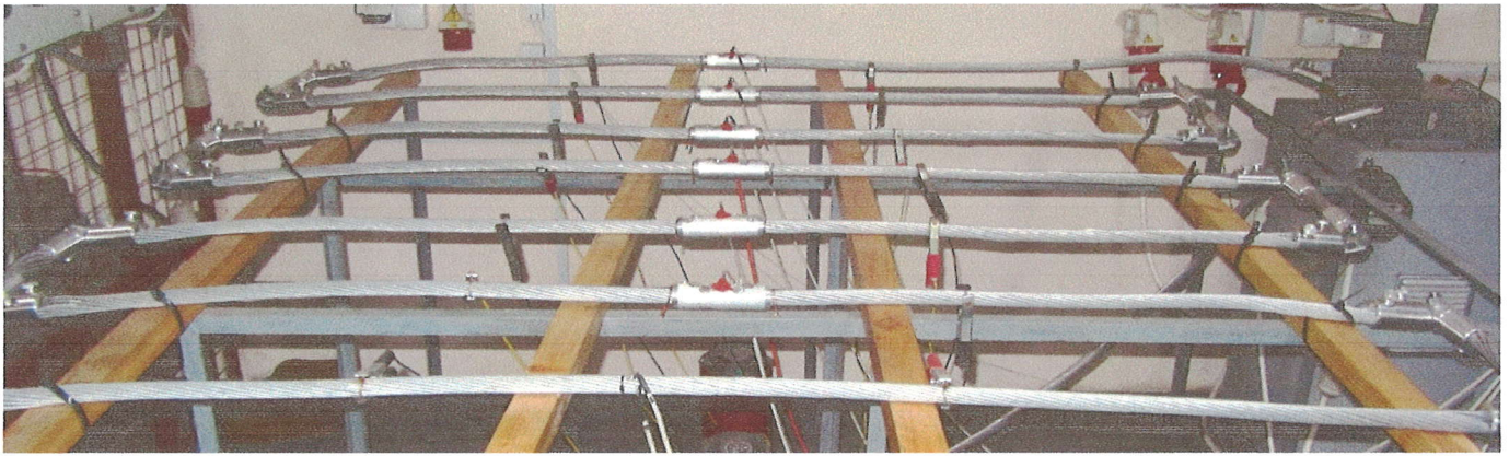
Fig.5 – The connectors during the tests in the circuit with maximum conductor's cross section 240 \text{ mm}^2 and a combination of aluminum – aluminum
