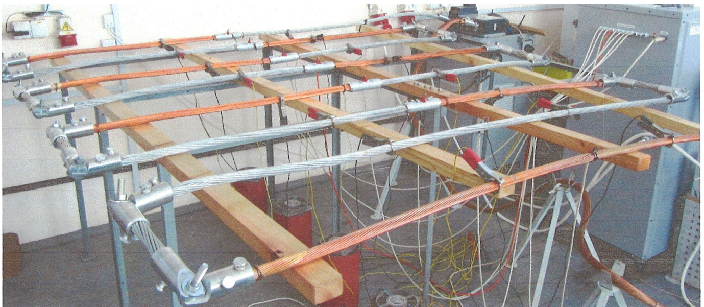
Fig.7 – The connectors during the tests in the circuit with maximum conductor's cross section 240 \text{ mm}^2 and a combination of aluminum – copper
